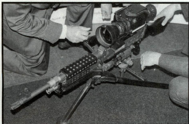
The FN M240B with prototype night vision sight. The sight is a new model derivative made by Litton.
