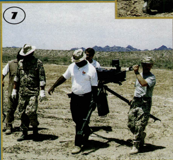
6. Next, Robert Hirt opens the cover and dumps a 40 mm ammo can full of water into the mechanism, then they slap another 32-round belt into the GMG and shoot it—no problem.
