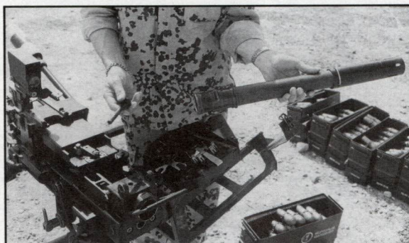
Barrel is removed by one pin that comes out after the top cover is removed.
