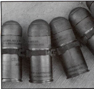
M918 TP 40 mm x 53 ammunition that was used in the test. On impact, it produces a bright flash, a report, and a puff of smoke.
