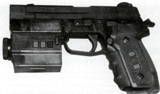
The Night Stalker integrated laser sighting system for SIG Sauer pistols manufactured by Wilcox Industries Corp. (formerly UIC Armament Corp.), pictured here with tactical flashlight. Laser sights are available in visible and infrared wavelengths (IR laser sights not available commercially). Flashlight module requires Night Stalker system for remote operation from custom grip. Control pad buttons preselect laser/flashlight and program laser pulse rate.
