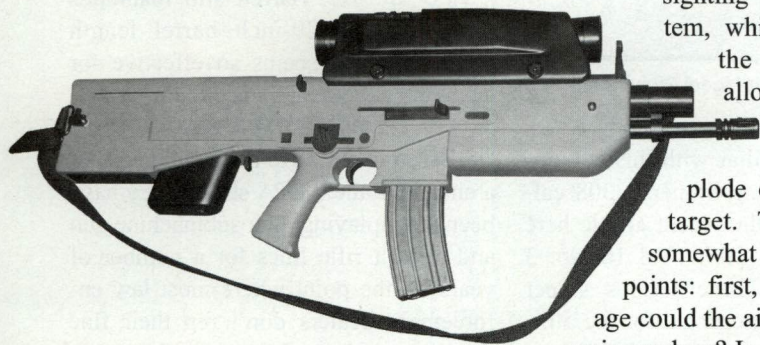
The Objective Individual Combat Weapon—sort of the ultimate over/under. On the bottom is a select-fire 5.56 mm rifle. On top, is a new 20 mm type launcher that has airburst arming out to 1000 meters.
